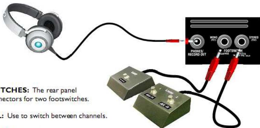
**FOOTSWITCHES:** The rear panel has jack connectors for two footswitches.
